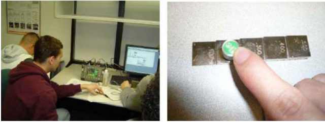
FIG. 11. (Color online) Calibration of the flaw detectors using a straight-beam probe.
