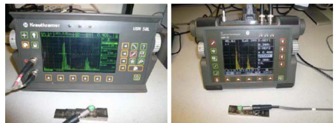
FIG. 10. (Color online) Portable ultrasonic flaw detectors USN 58L and USM 35X (from left to right).
